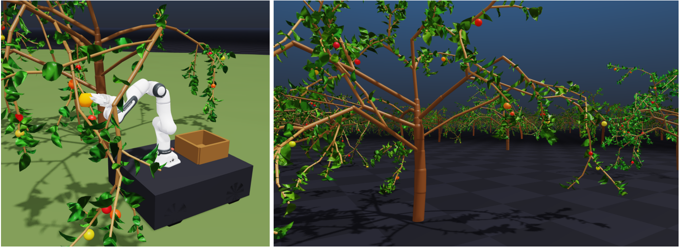
Fig. 1: ORCHARDBENCH . A physically-grounded, GPU-parallel apple orchard. Left : a mobile manipulator (Clearpath Ridgeback base and Franka arm) autonomously harvesting a compliant, fruit-bearing tree over bumpy terrain—here holding a picked apple beside the collection bucket, amid foliage that moves with the branches. Right : one hundred domain-randomized trees simulated in parallel, each a distinct plausible tree grown by a stochastic L-system, varying in growth habit, foliage, fruit and colour. Branches snap under load and apples detach at realistic pull forces (Section IV).
